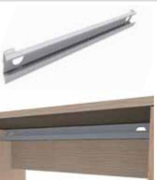
1.5 mm thick cold laminated steel sheet metal beam. Finished with 100 micron epoxy paint, polymerized at 220° C. "C" shape section, opened to the inner side of the desk to allow the cable management.
