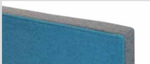
16 mm thick particle board base with both sides upholstered over a 5 mm thick foam, fixed to the framework by specific fittings. Sewings at laterals.
